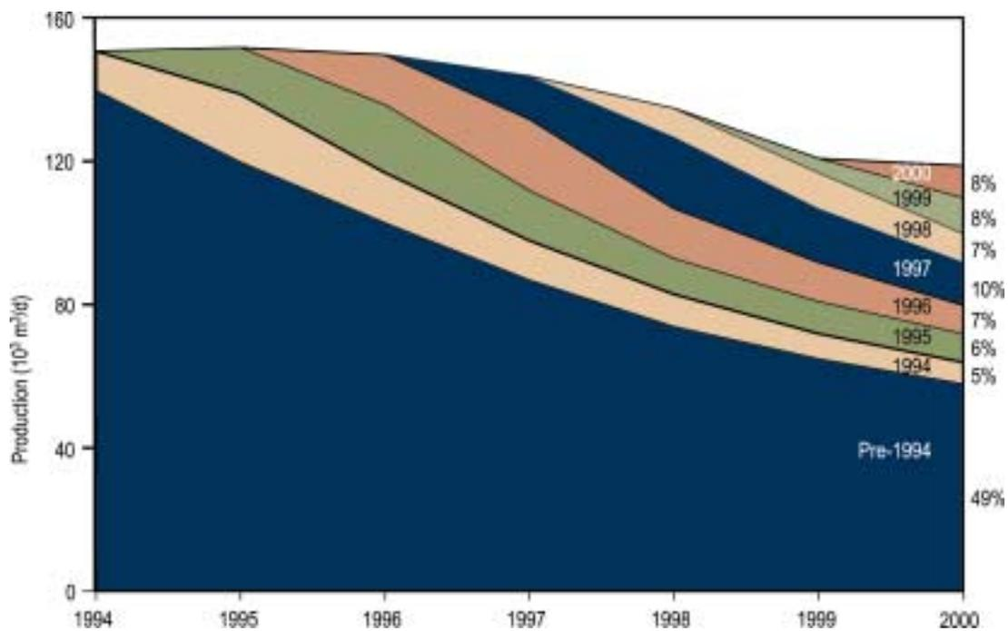
Figure 3.11. Total conventional crude oil production by drilled year
