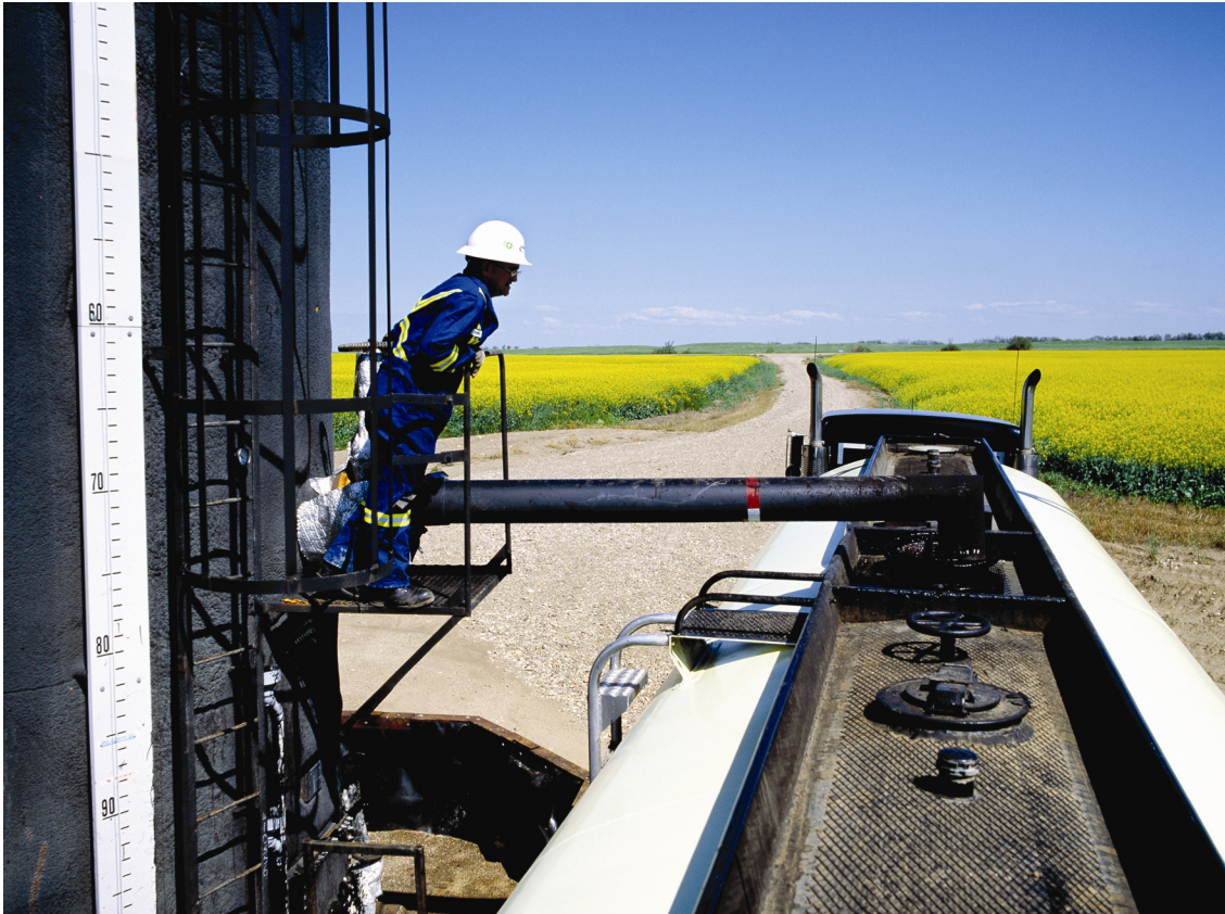
Loading oil into truck from tank farm
