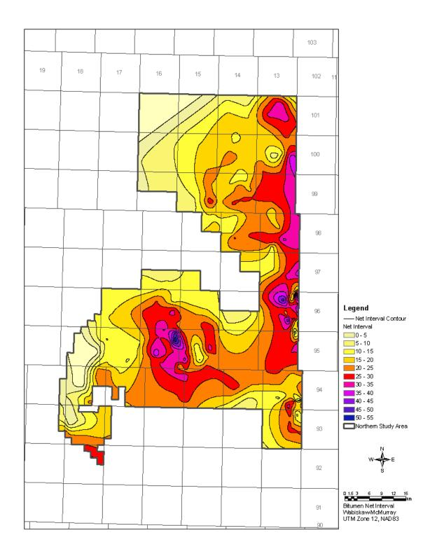
Figure 85 – McMurray Channel, Wabiskaw D Sand, Wabiskaw C Sand, Wabiskaw A Sand Bitumen Isopach
