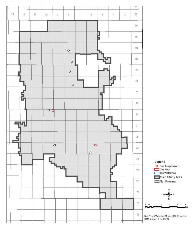
Figure 56 – McMurray B2 Channel Gas/Top Water Map with B2 Channel Distribution
