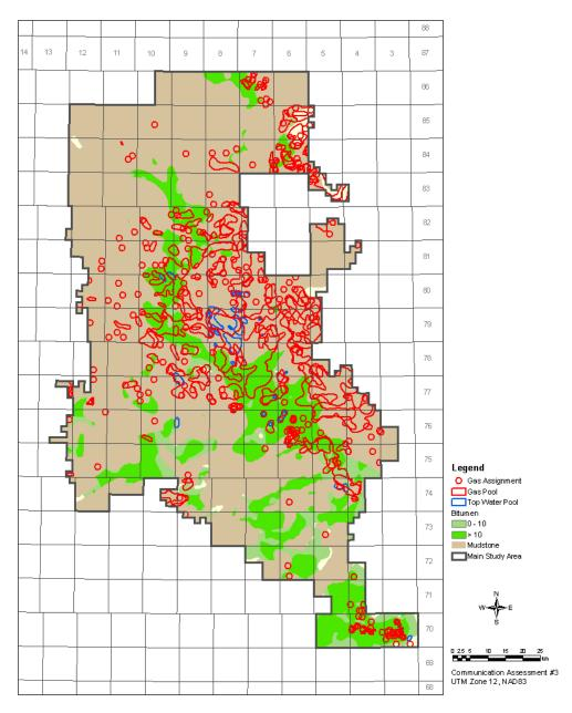
Figure 95 – Case 3, Gas / Top Water above McMurray A2 Mudstone and McMurray Channel Bitumen
