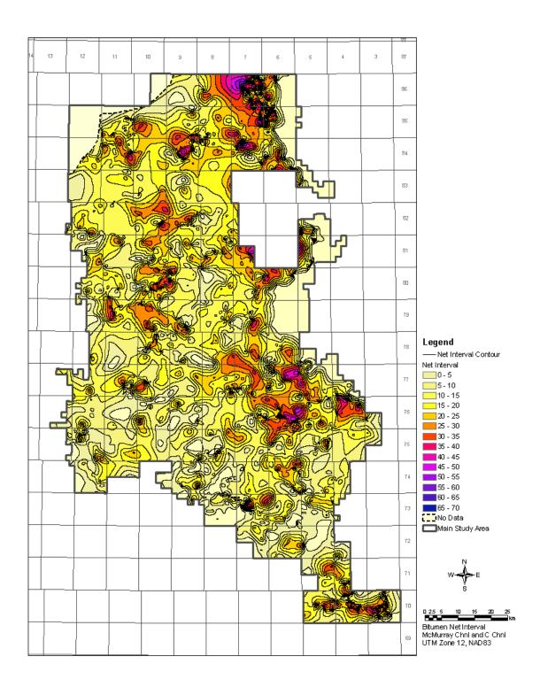
Figure 72 – McMurray C Channel / McMurray Channel Bitumen Isopach Map
