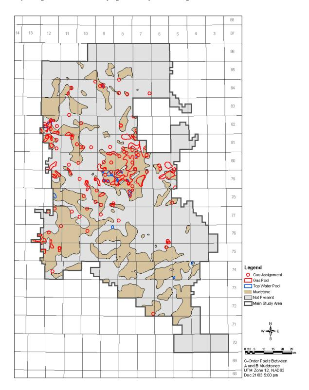
Figure 59 - Composite McMurray B Gas / Top Water with B2 Mudstone Distribution
