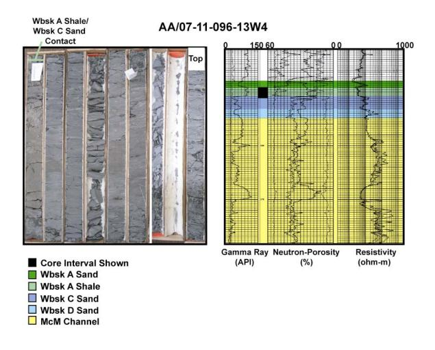
Figure 43 – Wabiskaw A Shale Core Photo and Well Log
