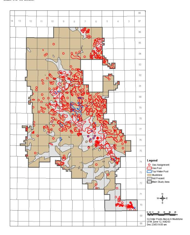
Figure 65 – Composite of Gas / Top Water above A2 Mudstone with A2 and B2 Mudstone and D Shale Distribution
