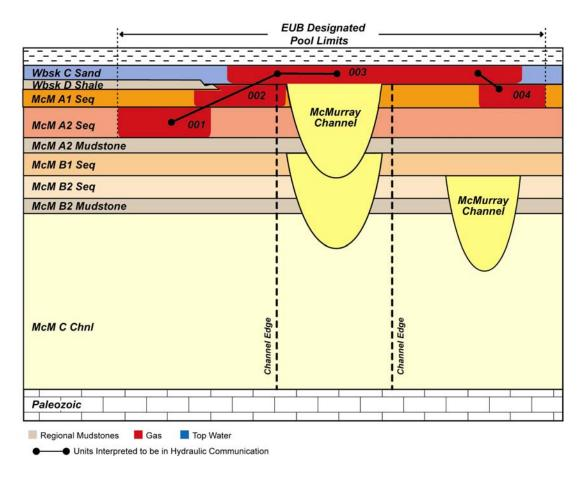
Figure 52 – Schematic Illustrating Individual Gas Accumulations and Corresponding EUB Designated Pool
