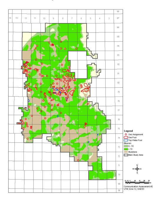
Figure 92 – Case 2, McMurray B Gas / Top Water and McMurray Channel Bitumen
