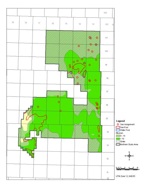
Figure 106 – Case 6, Wabiskaw C Sand Gas / Top Water and McMurray Channel / Wabiskaw D and C Bitumen
