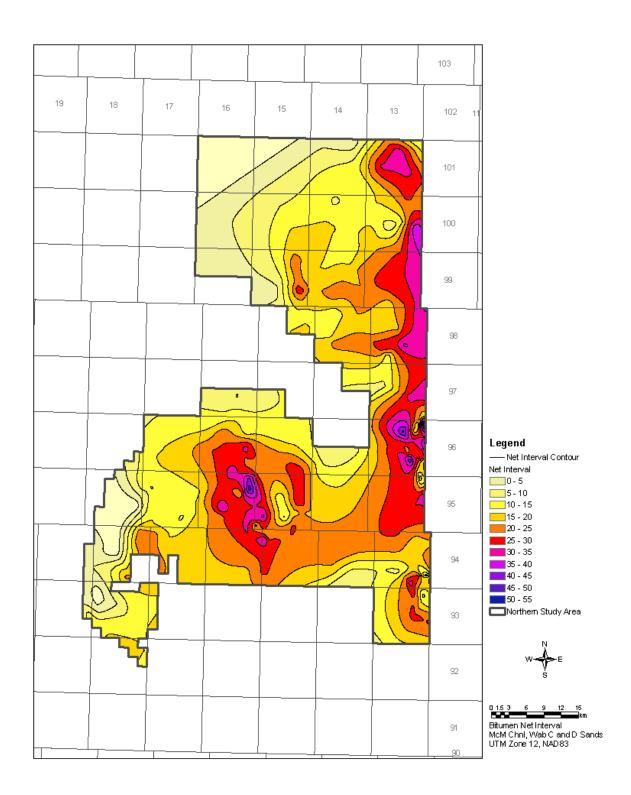
Figure 83 – McMurray Channel, Wabiskaw D Sand, and Wabiskaw C Sand Bitumen Isopach
