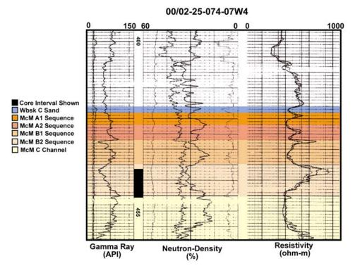
Figure 10 - McMurray B2 Sequence Core Photo and Well Log
