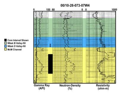
Figure 8 – McMurray Channel Core Photo and Well Log
