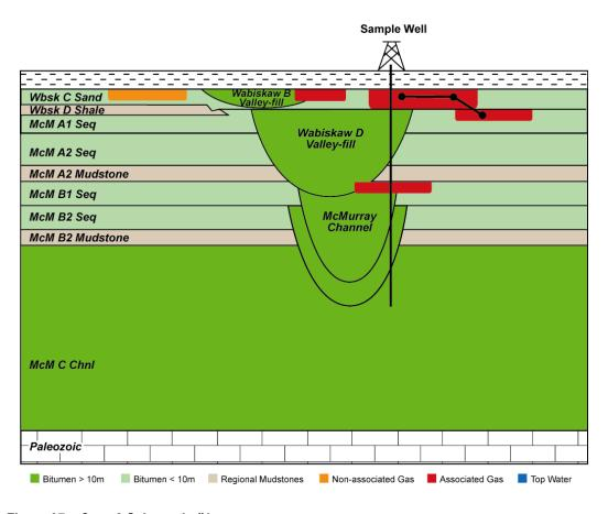
Figure 97 - Case 3 Schematic #1
