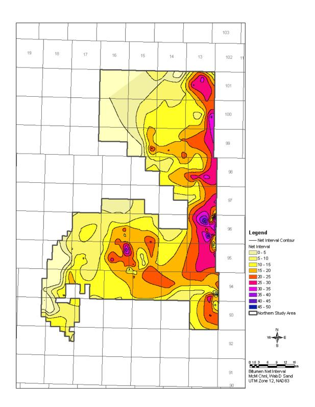
Figure 81 – McMurray Channel and Wabiskaw D Sand Bitumen Isopach
