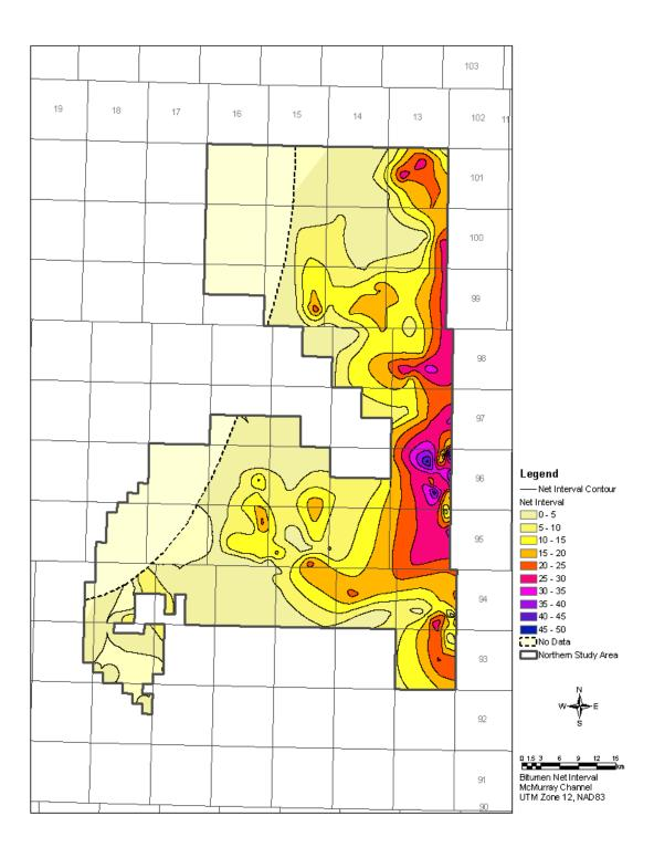
Figure 79 - McMurray Channel Bitumen Isopach
