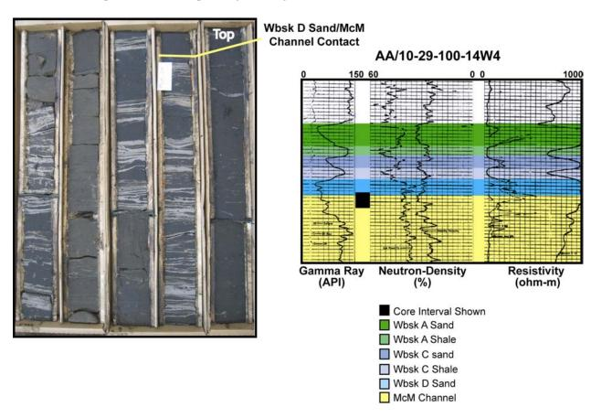
Figure 38 – McMurray Channel Core Photo and Well Log
