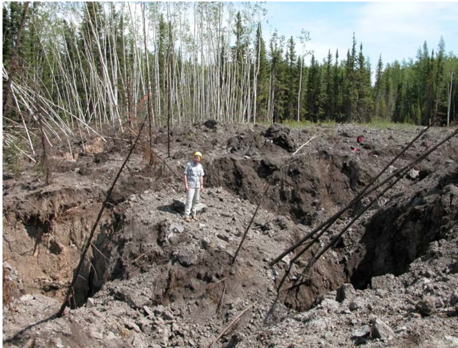
Photo 55: View to the east showing the main crater and a central plug of rock and soil, including trees, which was not removed during the initial steam release.
