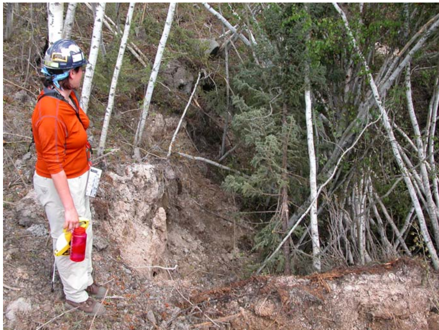
Photo 16: View looking north along the edge of the “sinkhole” feature, showing tilted, rotated soil blocks.
