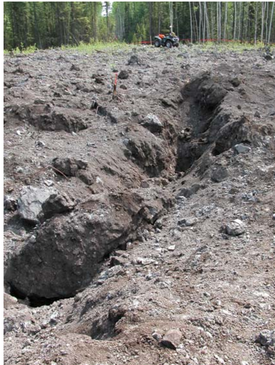
Photo 8: Collapsing “fracture-like” or trench feature that trends at 105° away from the main release crater/vent. 15.6 m in length.
