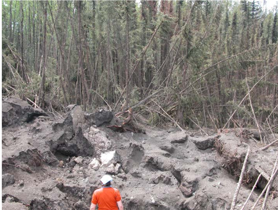
Photo 22: View looking south at the edge of the blast area, near the secondary release site. Note the tilting of trees to the east and west in this photo, and the uplifted till(?) cover with possibly grey Clearwater shale in the lower left centre of the photo.
