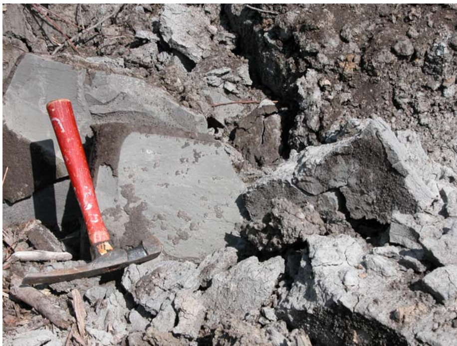
Photo 58: Projectile of grey-green Wabiskaw shale/siltstone, as identified by K. Stasiuk, found near the east side of the main crater.
