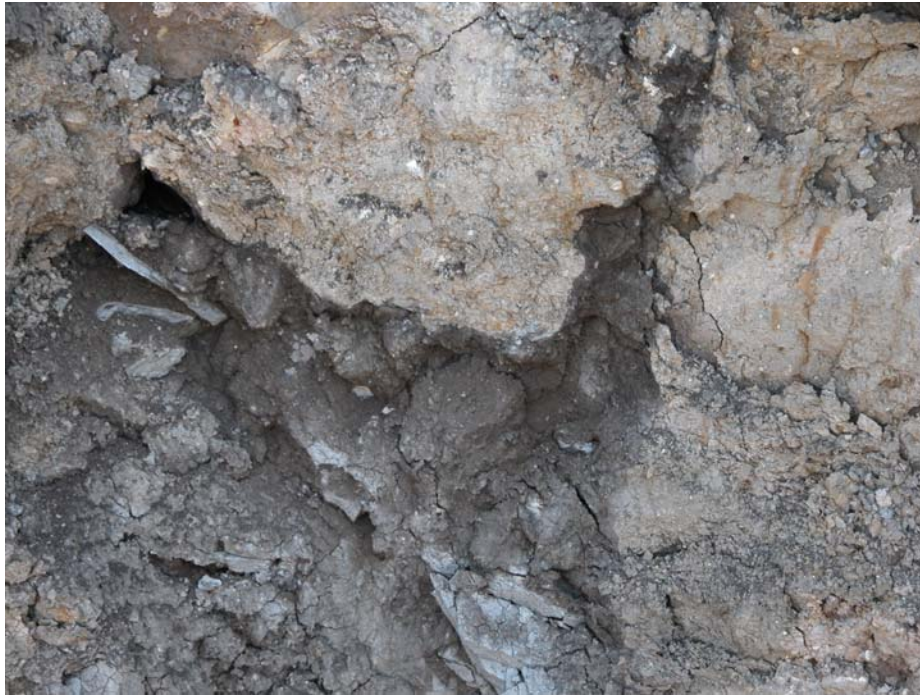
Photo 5: Close-up of the deformed rock along the main crater edge. Poorly cemented soil or rock in this area were damp and in one location, smelled strongly of oil.
