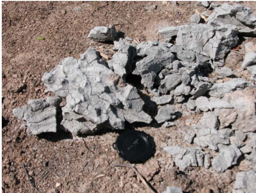
Photo 37: Close-up of a one shattered projectile of Clearwater shale, (Formation identified by K. Stasiuk, TOTAL). Projectiles in this location typically ranged from 5 to 25 cm diameter based on the volume of shattered material.
