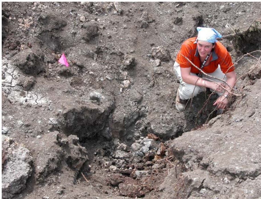
Photo 28: Close-up of the main steam release vent in Photo 27, showing discolouration in the soil. Station 8.
