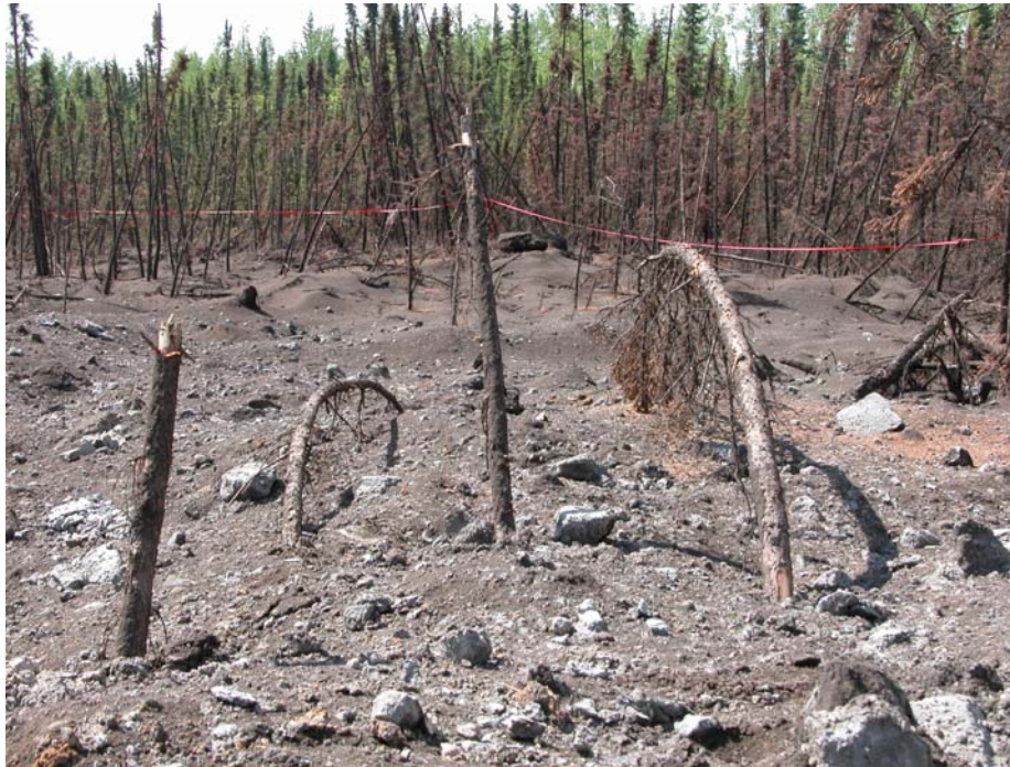
Photo 33: View to the south from the main crater showing trees bent over From the initial blast and sediment loading.
