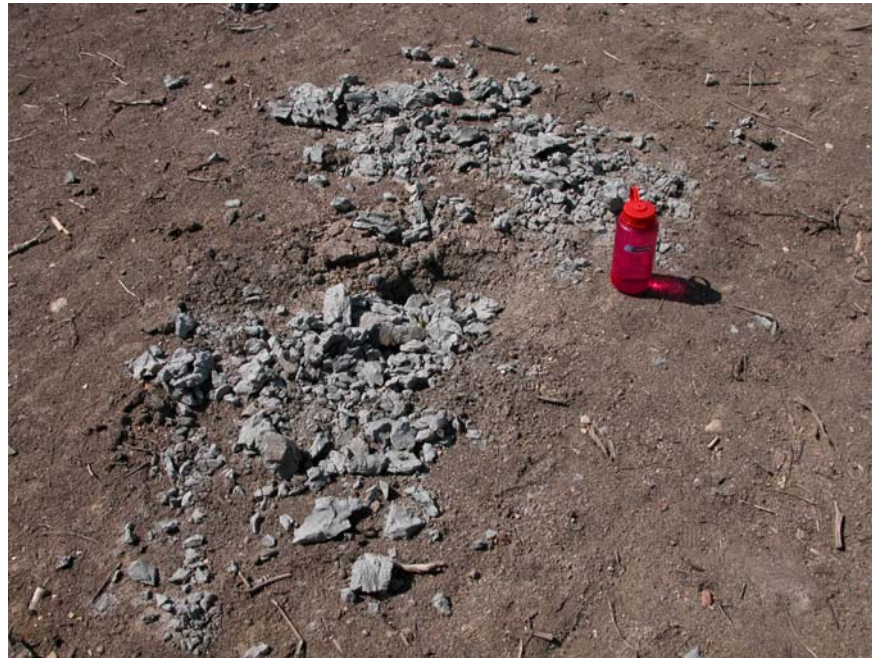
Photo 36: Shattered projectiles of grey Clearwater shale along side the road to the plant, adjacent to the pipeline. Eight projectiles were counted within a 16 m 2 area at this location. The impact shattered most blocks with some blocks embedding a few centimetres into the clay/silt ground surface. Additional projectile blocks were noted on the other side of the road. This station is approximately 300 metres west of the main steam release crater.
