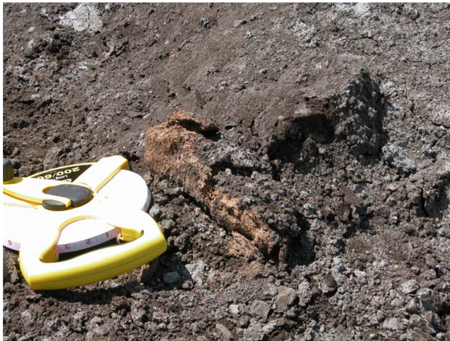
Photo 34: Close-up of fibrous peat moss that appears to have been transported in the air from a nearby location.
