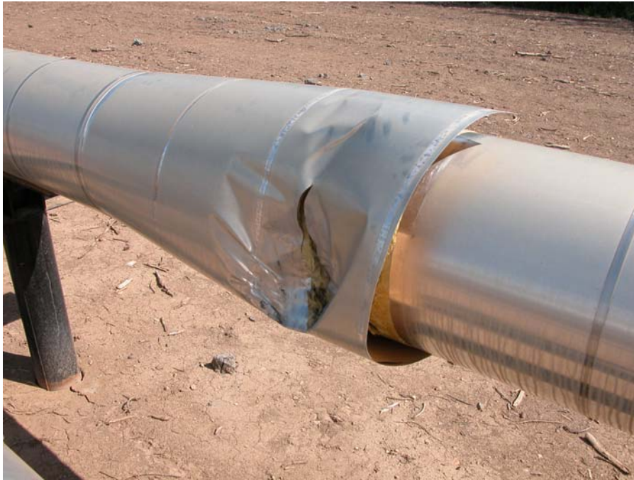
Photo 39: Close-up of damage to a surface pipeline which was struck by a rock projectile. The impact was on the top and west side of the pipeline indicating the block that did the damage must have had a fairly vertical trajectory.
