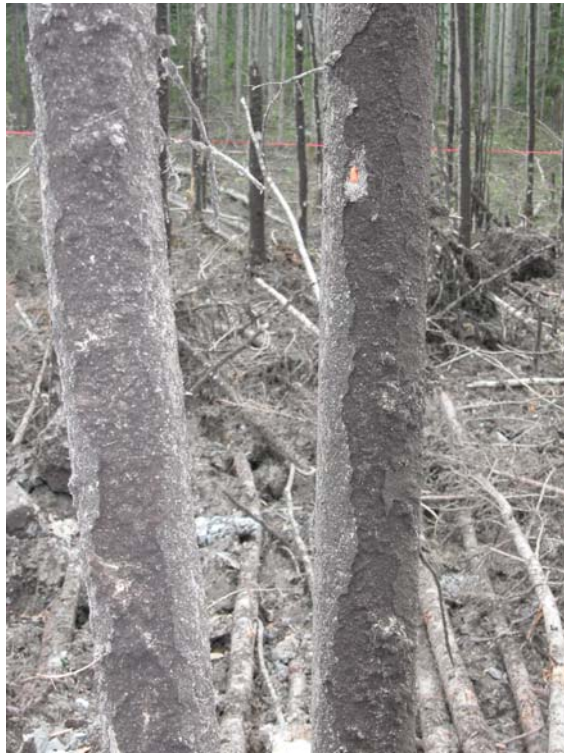
Photo 45: Soil coating of 1-2 cm on trees, indicating main blast direction.
