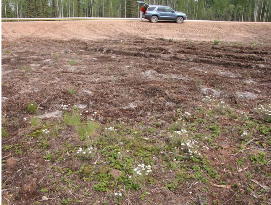
Photo 41: View looking east across the road to the plant showing small disintegrating grey shale (Clearwater?) projectiles which must have travelled horizontally in excess of 300 metres. These appear to be the furthest that projectiles travelled.
