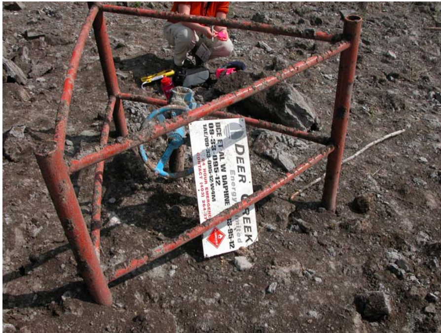
Photo 53: Relatively undamaged wellhead at 0/09-33.
