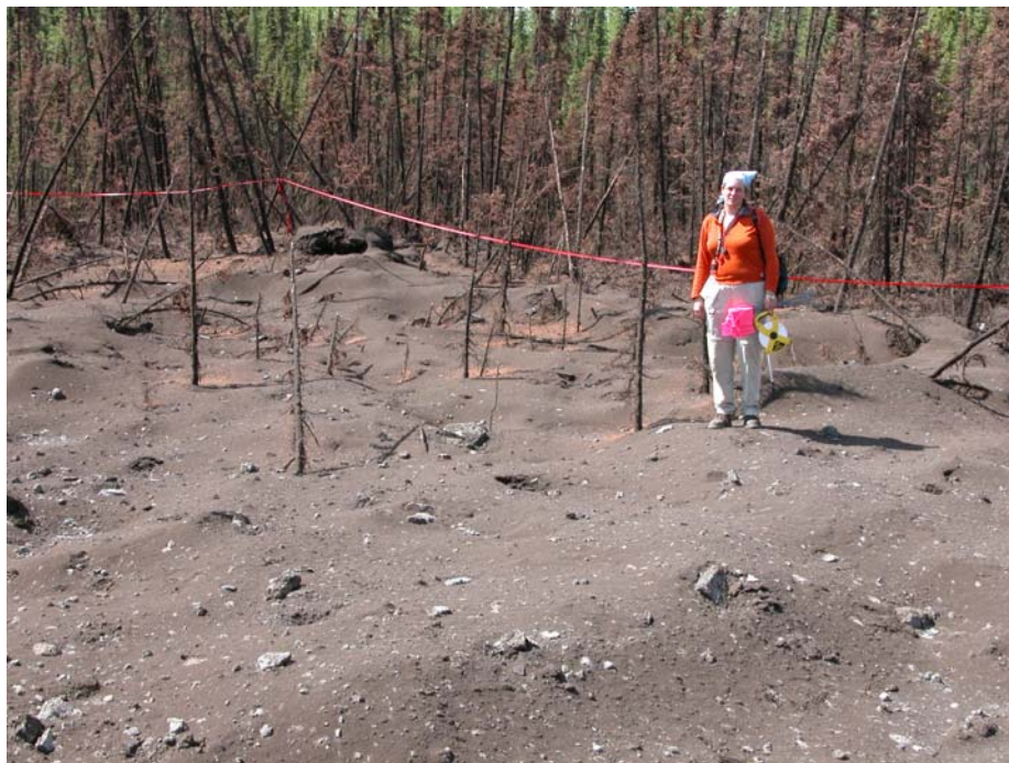
Photo 32: View to the west edge of the blast area showing a cover of airborne silt overlying and mixed with shale? bedrock projectiles.
