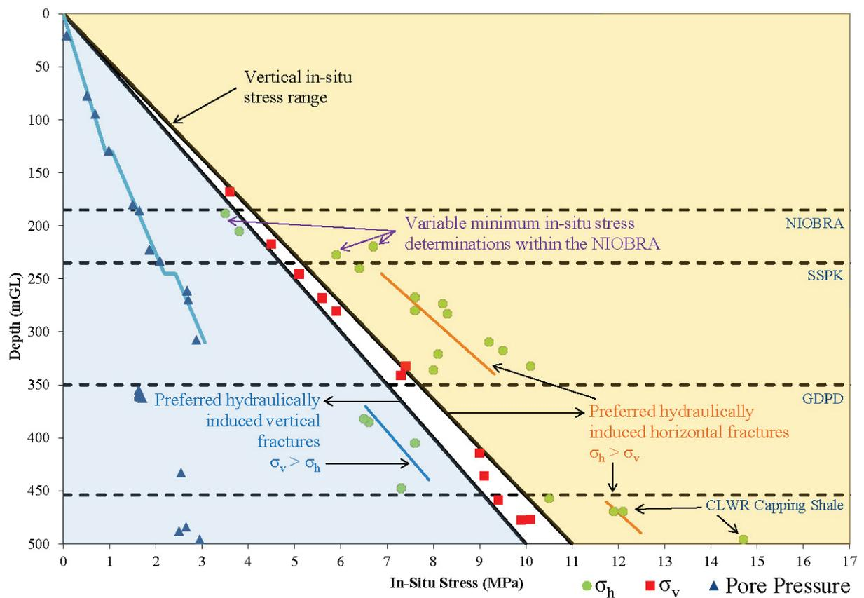
**Figure 17. Pore pressure and in situ stresses in PAW (from CNRL 2015, figure 3.1-8). This figure provides a basis for understanding the expected fracturing of the formation associated with injection pressures in relation to the stress gradients.**
