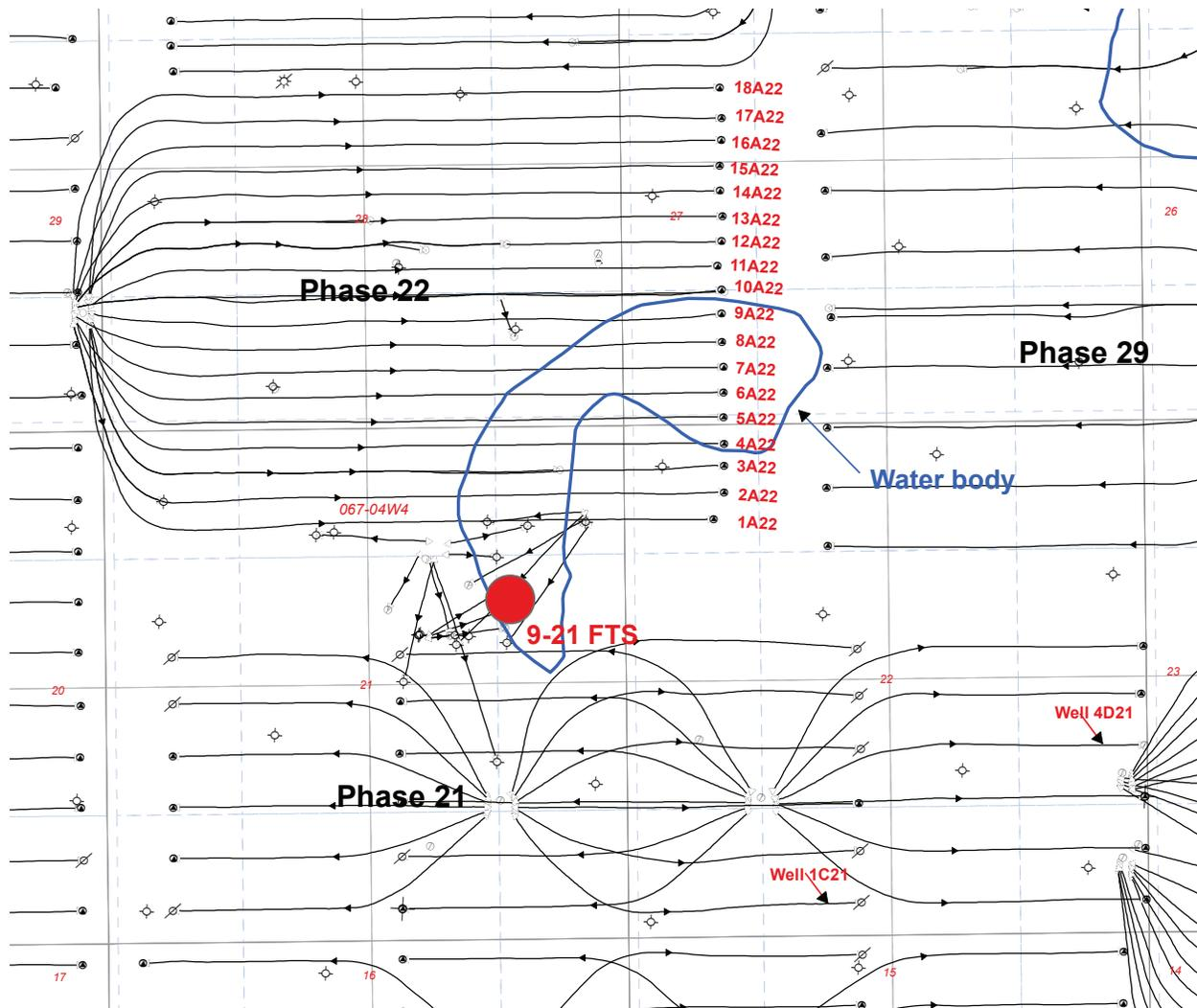
**Figure 8. Surface bitumen emulsion release at 9-21 FTS site.**
