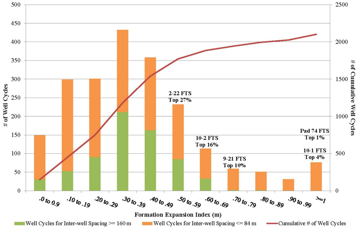
Figure 20. Primrose FEI distribution with FTS events in the highest 27% on per-well basis (from CNRL 2015, figure 1.3-4).
