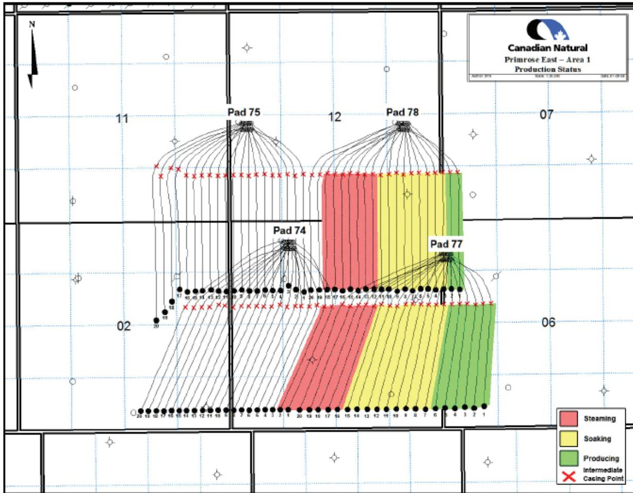
Figure 5. Primrose East Area 1 well operation status on January 2, 2009 (from AER 2013, figure 4).
