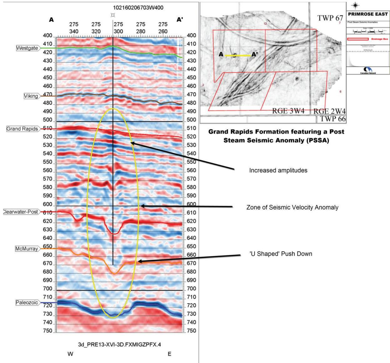
Figure 13. Seismic cross-section of the 16-02-067-03W4 PSSA (from CNRL 2015, figure A.10-43). The figure illustrates a cross-sectional view of a vertical bitumen emulsion column saturated with natural gas migrating upwards from the Clearwater reservoir and through the Grand Rapids Formation as observed on the 4D seismic profile.
