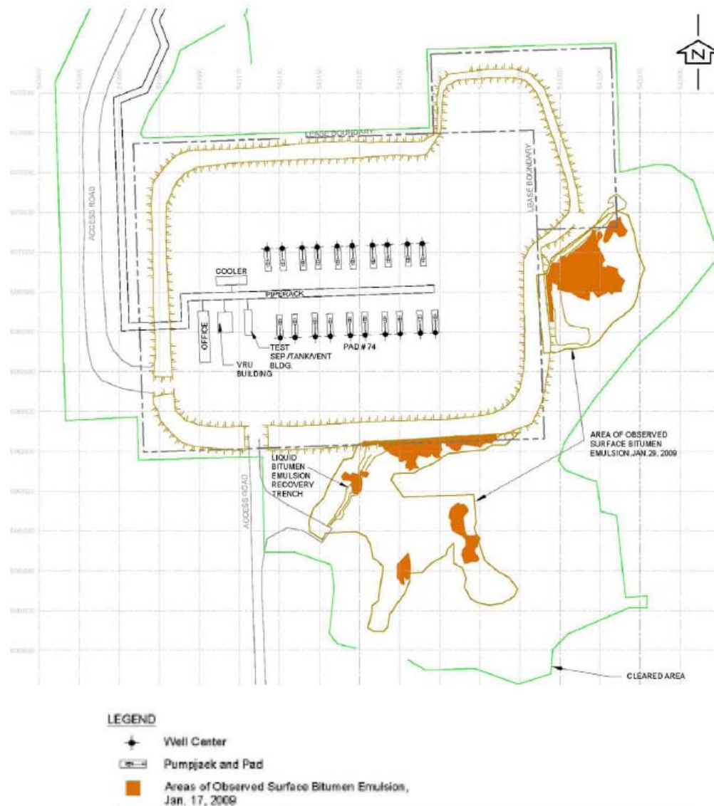
Figure 3. Schematic of Pad 74 showing the location of the bitumen emulsion releases
