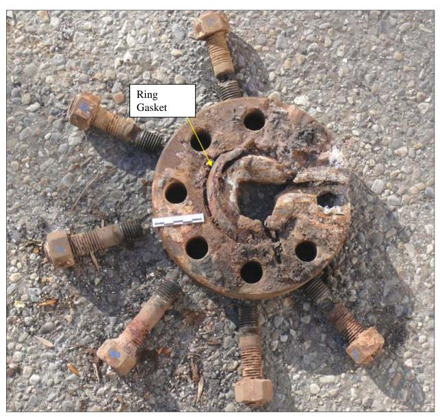
Figure 2. Exposed blind flange
