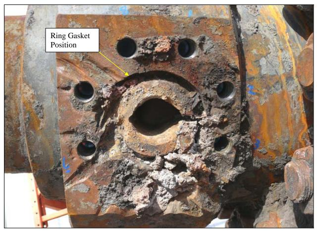
Figure 3. Casing bowl sealing faces
