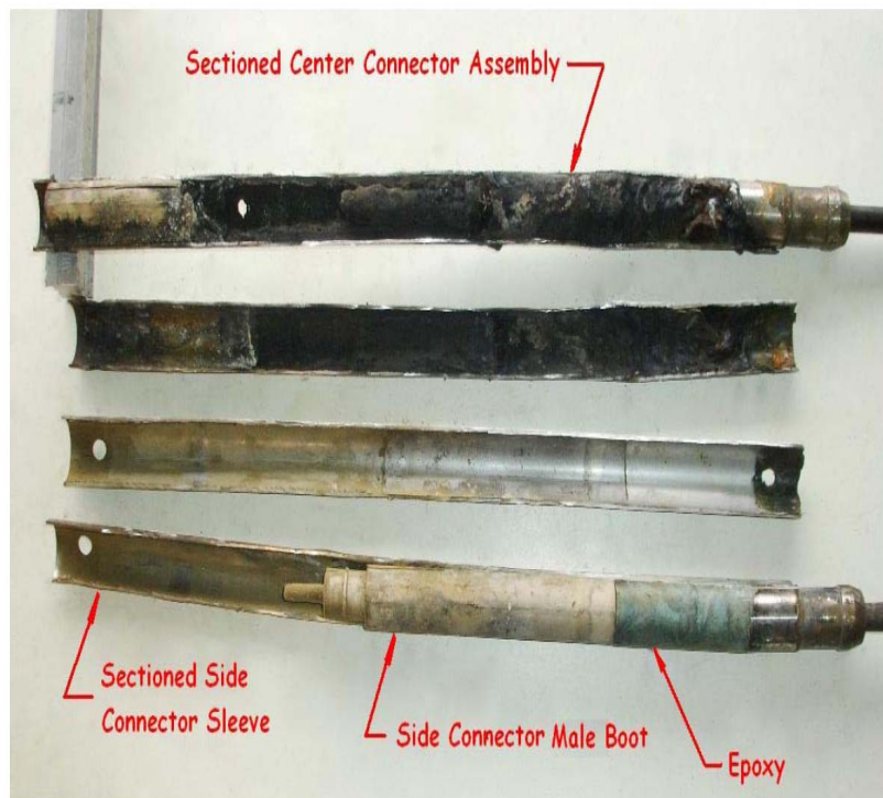
Figure 4. Comparison of damaged connector vs. undamaged connector
