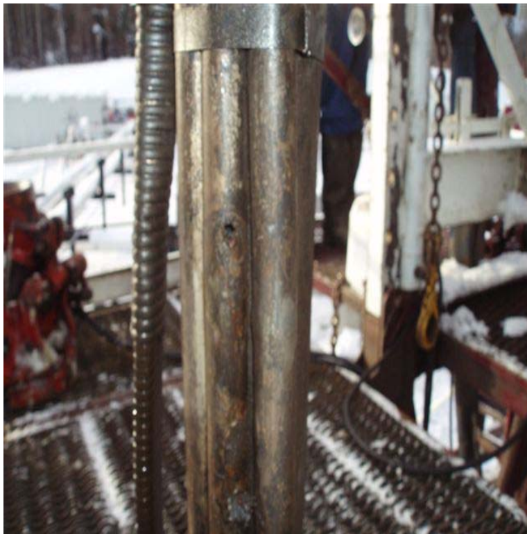
Figure 3b. External damage to connector assemblies
