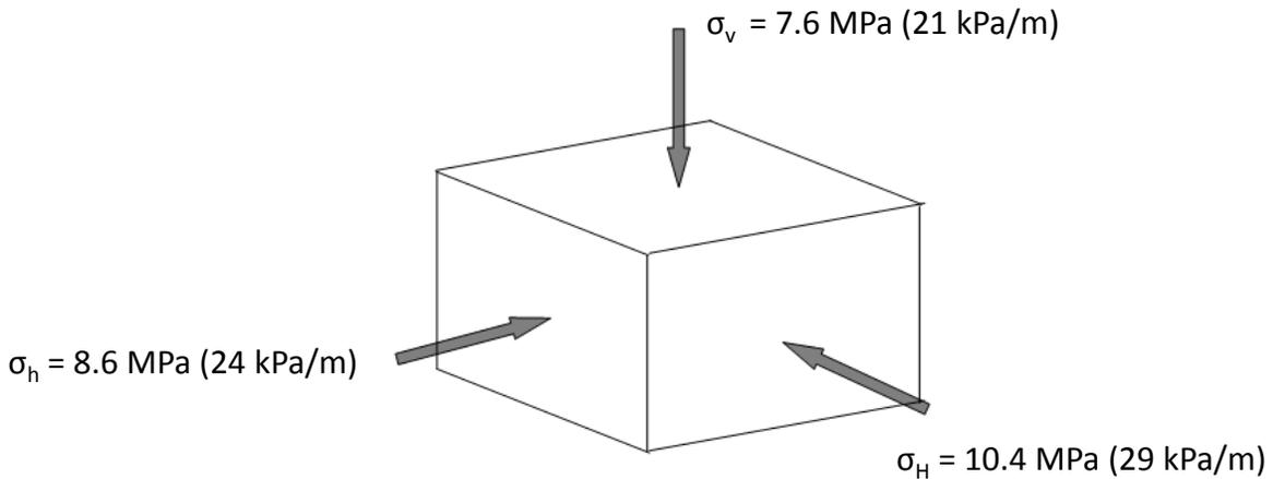
**Figure 6-2** Example of Typical Principal Stresses in the Joli Fou Formation at a depth of 360 m
