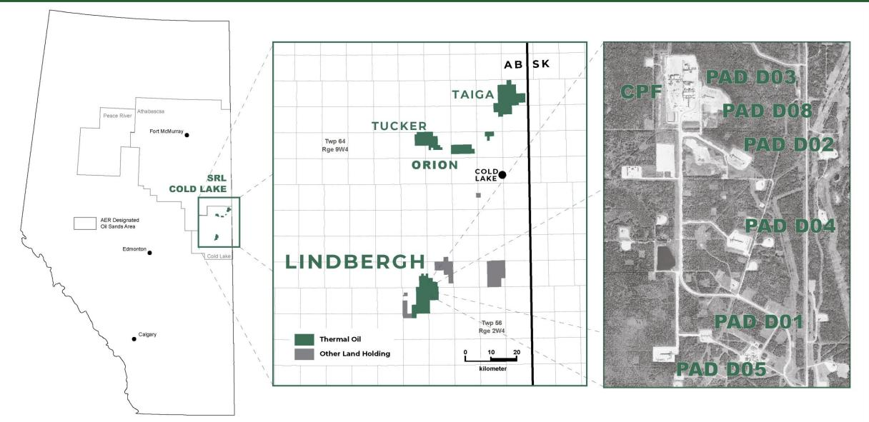
Lindbergh is an in-situ oil sands steam-assisted gravity drainage (SAGD) project consisting of a central processing facility (CPF) and six well pads situated in 04-25-058-05W4M, approximately 30 km south-east of Bonnyville, Alberta.
