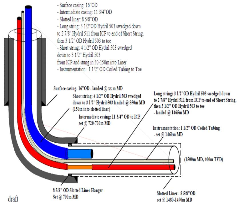
□ 2 injectors have been reconfigured with a single injection string with multiple steam splitters.
