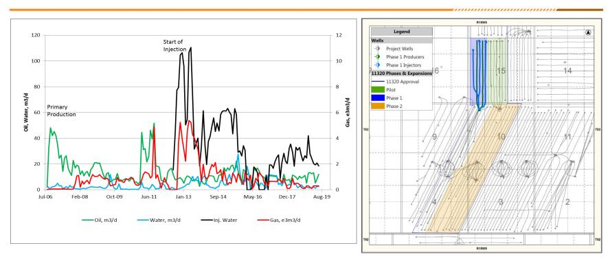
Phase 1 consists of 2 injectors and 2 producers
