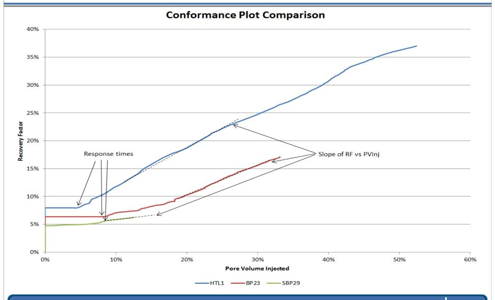
Plot showing Recovery Factor (RF) versus Pore Volume (PF) Injected. Indicates effectiveness and performance of the flood.
