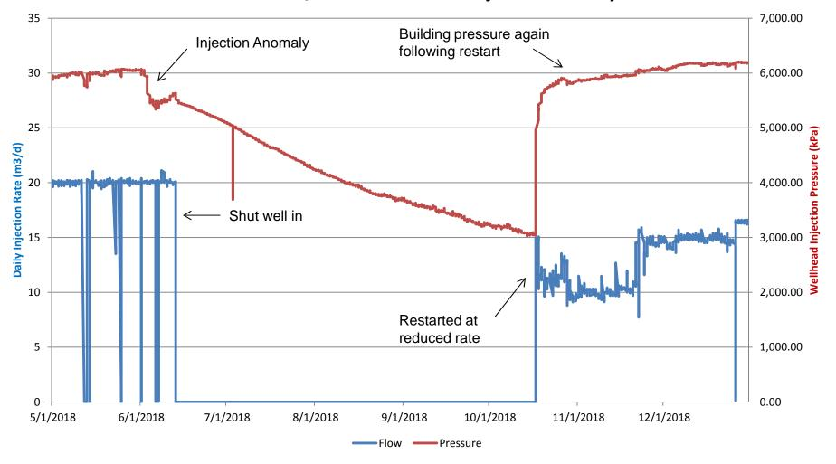
**00/16-31-082-21W4:** Injector was shut in shortly after anomaly to allow time for the dilation to "heal". Restarted at a reduced rate and found pressure has built back up to pre-dilation levels.
