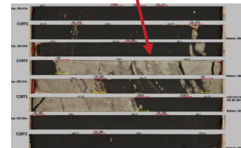
AC050B: Steam chamber development above mudstone in September; 1 to 2 m mudstone acted as a baffle, not barrier, to flow
