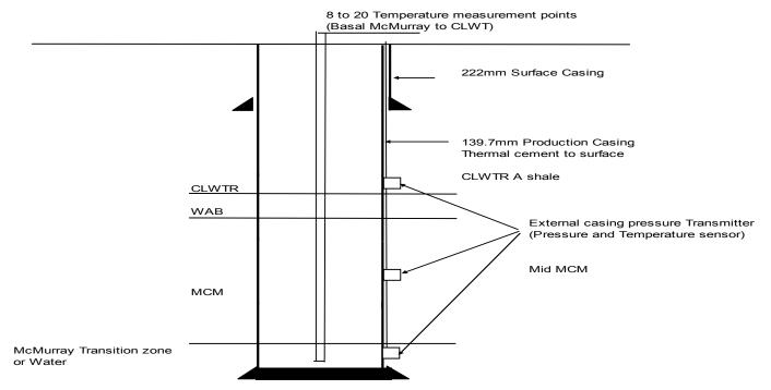
Note: Shows a plan for 2011-2013 drilled observation wells, as previous wells don't have external casing transmitters
