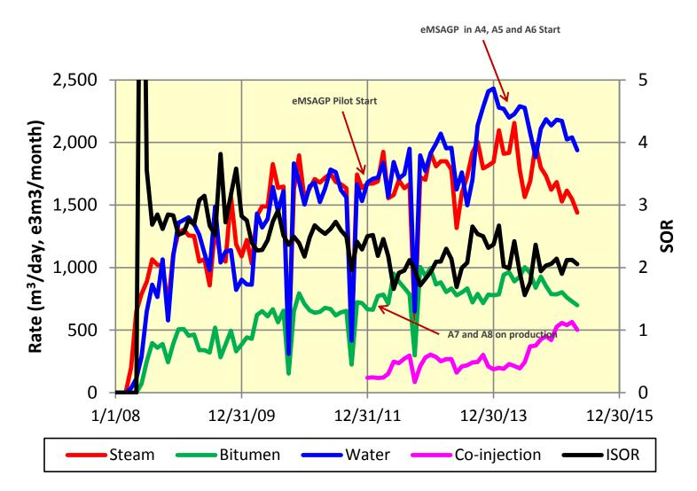
Increased water to steam ratio noted recently was mostly from two edge SAGD well pairs (A6 and A8), a result of edge or bottom water incursion
