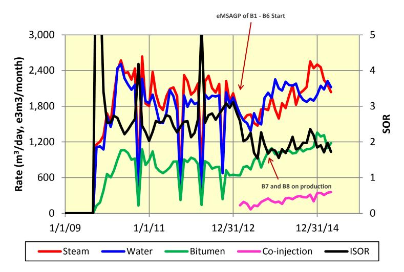
Increased steam injection rate was to increase the steam chamber pressure in two SAGD well pairs (B1 and B2) that have bottom water
