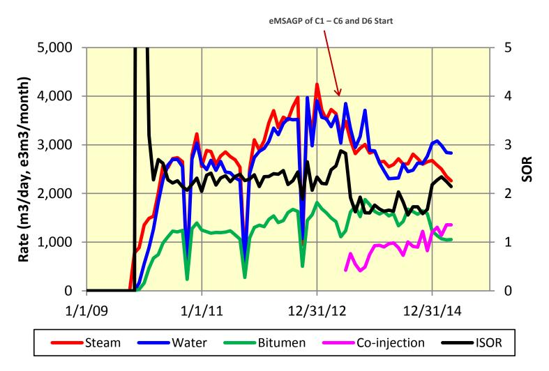
Bitumen production drop in December 2014 was partially due to measurement calibration
