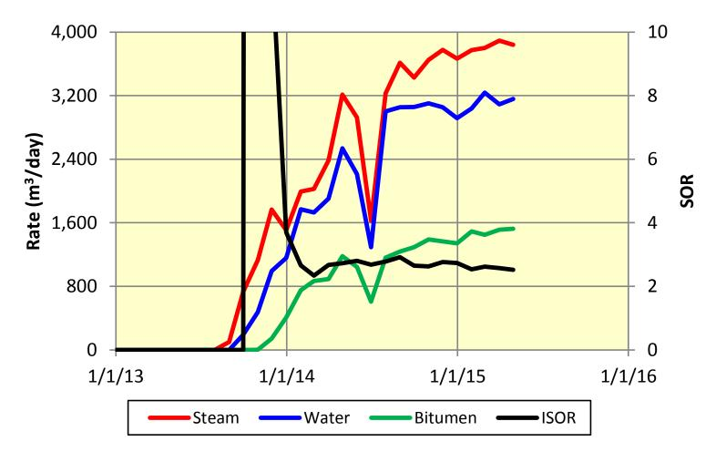
M9P and M10P have low TFSR due to poor producer inflow, lowering the overall WSR. Both wellpairs operate at low pressure so steam is not considered lost to thief zones. Temporary steam reduction due to pipeline construction activity in mid-2014.
