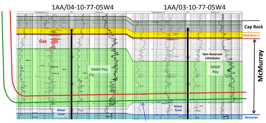
Bitumen / Water Contact
