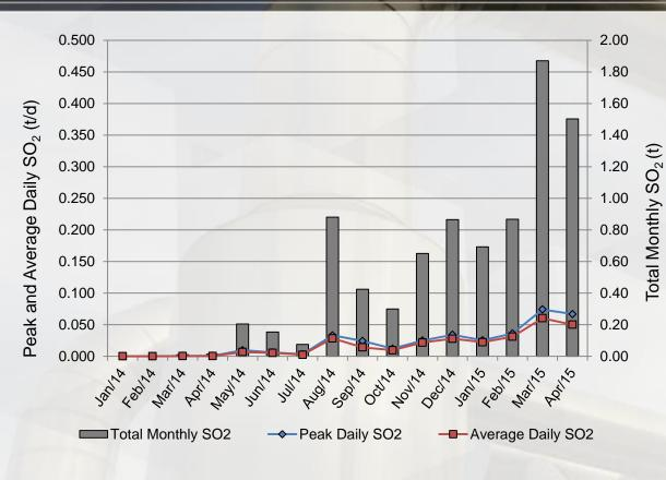
Total Emitted  $SO_2$  = Boiler  $SO_2$  + Flare  $SO_2$
