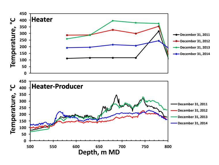
Thermocouple data used to monitor heater temperature as fiber readings have become unreliable.
