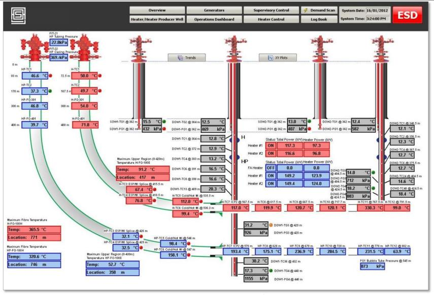
Instrumentation tied to central data acquisition system for remote real-time monitoring and control from the field and Calgary
