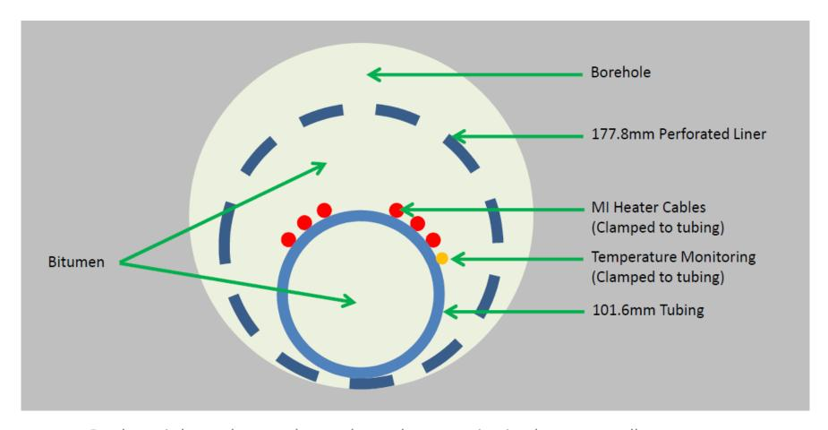
o Producer is heated to accelerate thermal communication between wells
