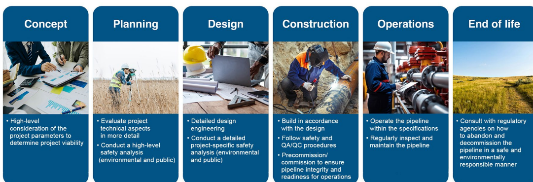
Figure 2. Heat distribution pipeline life-cycle phases
