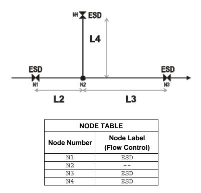
Finally, using the labelled schematic and the Node Table, the gathering system can be described in a larger table, as shown in this example. This table will be used for the inputs to the *ERCBH2S* **BATCH** page. Remember to keep both tables and the schematic for future reference.
