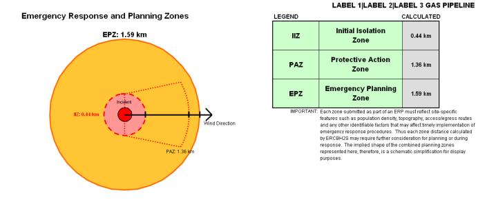
On the **ERP SUMMARY** page, the hazard zones are significantly reduced from the **NO MITIGATION** ESD instrumentation settings. These results may be advantageous from an emergency planning perspective and for general public safety. It remains to be examined by the operator if the normal fluctuation of pressure through the pipeline segment (due to process or load fluctuations) may trigger false ESD closures.
