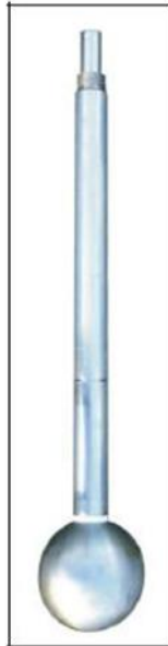
Figure B-3: Flow Penetrometer Rod with Ball Attachment
