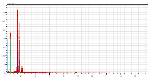
Figure D 129: An EDX analysis at point 4. The mineral in the center is kaolinite with calcite surrounding it. An SEM image showing this point precedes this EDX section.
