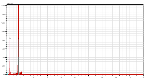
Figure D 128: An EDX analysis at point 3. The mineral is quartz.
