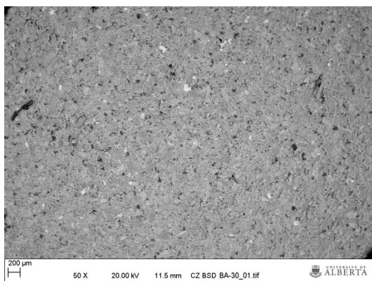
Figure D 111: A 50X magnification of Sample EN-30. At this scale, the sample appears relatively homogeneous although composed of a number of different minerals.
