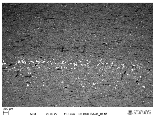
Figure D 120: A 50X magnification of Sample EN-31. At this scale, the layering can be clearly seen.
