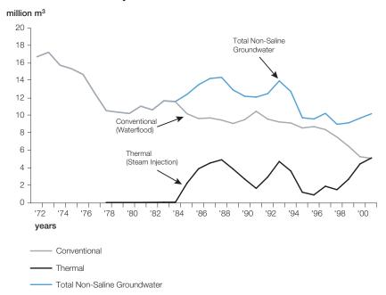
Since the mid 1970s, the use of non-saline groundwater and surface water for conventional oilfield injection has been declining in Alberta overall. However, uses for thermal oil recovery are expected to increase due to rapid expansion of the oilsands and heavy oil sectors.
