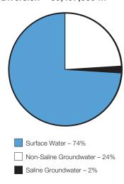
2001 Oilfield Injection Total Volumes – Source Water Total Diversion = 47,525,748 m<sup>3</sup>
