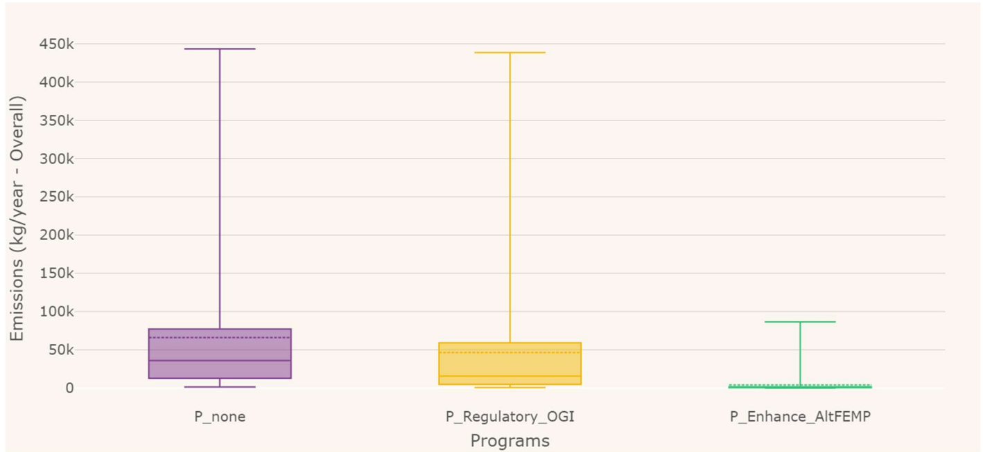
Figure 6. Box plots of daily emissions for the different program simulated considering the 16 sites in scope. Comparison of programs based on the Enhance Qube-based Alt-FEMP (P_Enhance_AltFEMP), FEMP routine OGI inspections defined by Directive 060 (P_Regulatory_OGI) and annual emissions in the absence of an LDAR program (P_none). On average, the Alt-FEMP program leads to greater emissions reductions than the D060 OGI-based program.
