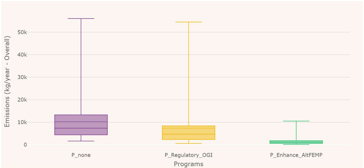
Figure 9. Emissions distribution sensitivity analysis - Box plots of daily emissions for the different program simulated considering the 16 sites in scope and leak rate distribution based on data from Ravikumar et al. 2020. Comparison of programs based on the Enhance Qube-based Alt-FEMP (P_Enhance_AltFEMP), FEMP routine OGI inspections defined by Directive 060 (P_Regulatory_OGI) and annual emissions in the absence of an LDAR program (P_none). On average, the Alt-FEMP program leads to greater emissions reductions than the D060 OGI-based program.
