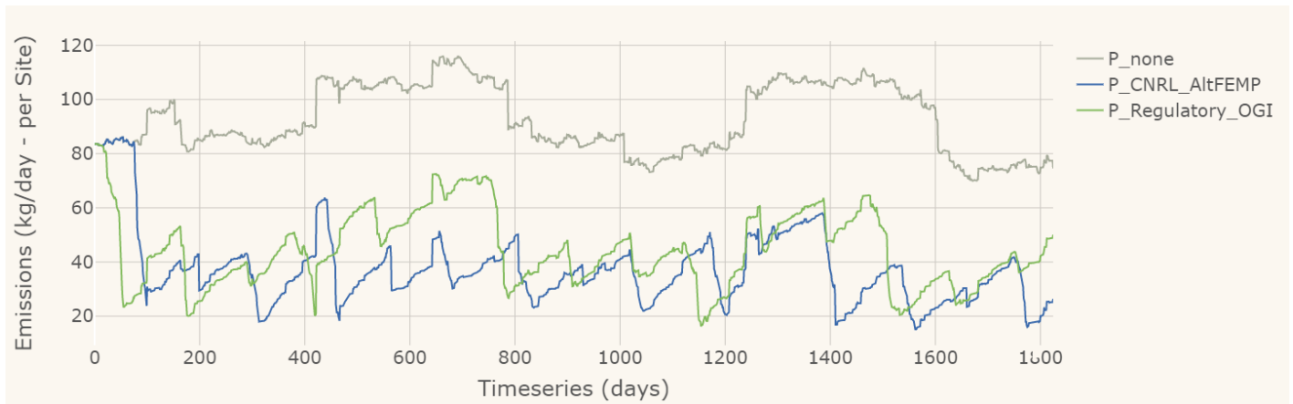
Figure 8. Timeseries of average emissions in kg CH 4 per site per day (averaged across all Alt-FEMP sites in simulation). Comparison of programs based on the Canadian Natural NW AB Alt-FEMP (P_CNRL_ALT_FEMP), base FEMP routine OGI inspections defined by Directive 060 (P_Regulatory_OGI) and annual emissions in the absence of an LDAR program (P_none). The cyclicity of the various time series is indicative of the dominant annual survey/screening requirements of the modeled programs with the Alt-FEMP (P_CNRL_ALT_FEMP) program showing biannual cyclicity as most sites have this requirement (as opposed to triannual) and the base FEMP program (P_Regulatory_OGI) showing annual cyclicity as most sites have this requirement (as opposed to triannual).
